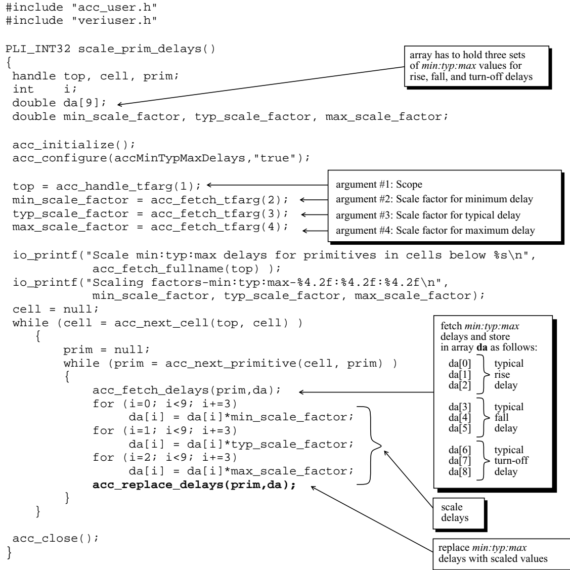
Figure 151—Using acc_replace_delays() in min:typ:max delays mode
